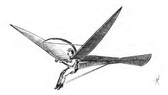
A hinged tail of an inverted trough form is attached to the rear of the frame, and may be actuated by cords attached to the feet of the aëronaut.
